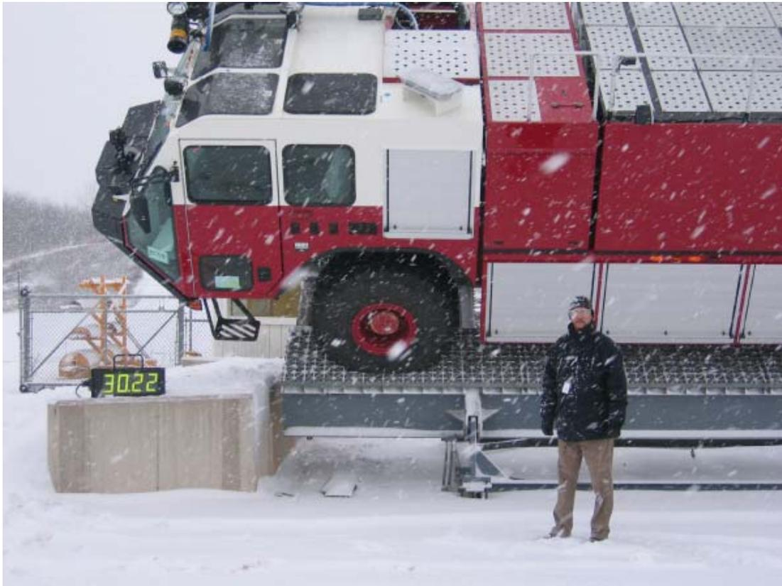
Mr. George Hall, HQ AFCEA/CEXF (AF Fire Protection Office) observing the 30 degree tilt table test for the AF's newest Crash Truck - the Oshkosh TI-3000 in Oshkosh WI. George conducts first article testing for every type of fire truck bought by the AF.
